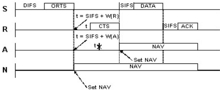
**Figure 6 Contention-Based Handshaking**
