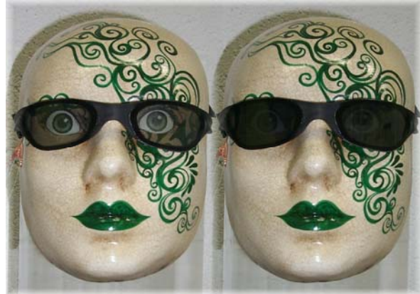
AlphaMicron's liquid crystal eyewear before and after switching the liquid crystal.
