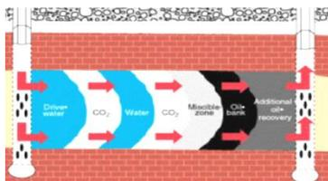
**Fig. 1:**WAG (Water Alternating Gas) involves alternating the injection of water & CO<sub>2</sub>. [7]
