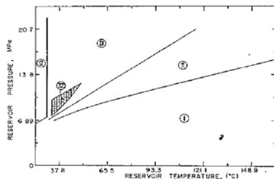
**Fig. 2:** The effect of reservoir temperature and pressure on carbon dioxide injection recovery mechanism. [10]
