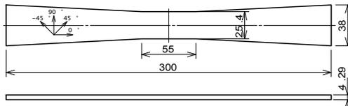
(a) NHT specimen for static tests
