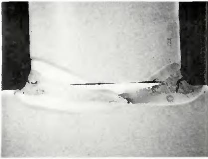
Fig. 10 — SAE 1045 cruciform welds with iron shim additions. Note the misalignment and cracks in the weld zone
