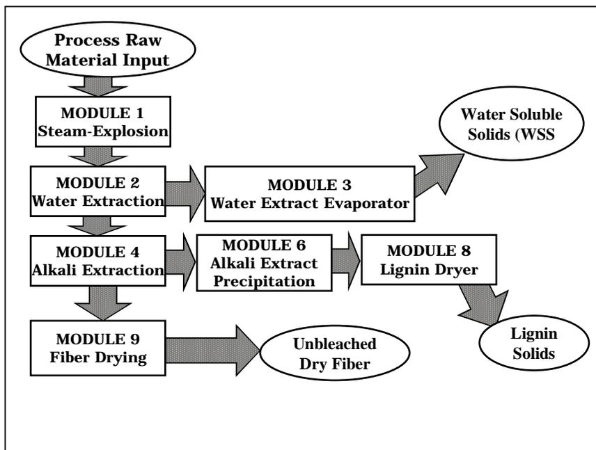
Fig. 8 Block flow diagram for scenario 3 - unbleached, extracted, steam-exploded fibers, wss concentrate and lignin precipitate (dry product)
