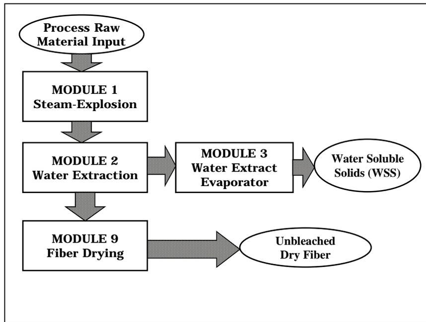
Fig. 7 Block flow diagram for scenario 2 - water extracted, unbleached steam-exploded fibers and WSS concentrate
