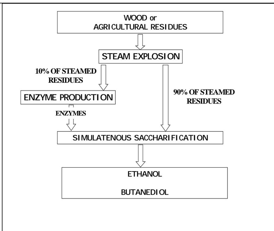
Fig. 3 A simplified process of biomass conversion to ethanol or butanediol using steam explosion and SSF according to E.K.C. Yu and J.N.Saddler
