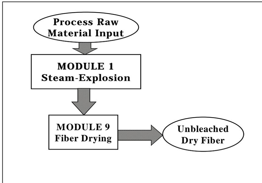
Fig. 6 Block flow diagram for scenario 1 - raw steam-exploded fibers
