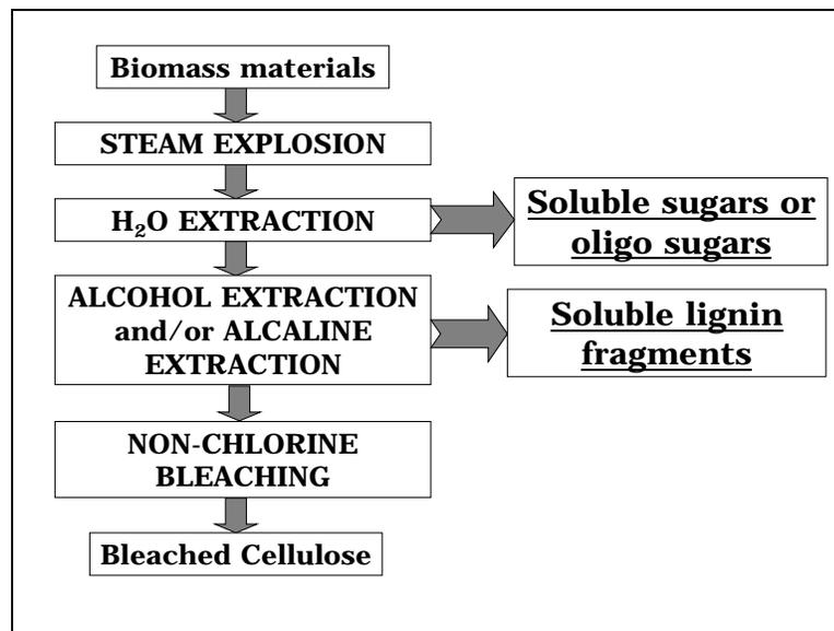
Fig. 5 Biomass materials refinery flow diagram in case of the steam explosion pretreatment
