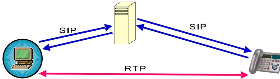
Illustration 1.3: Placing a SIP call through a proxy
