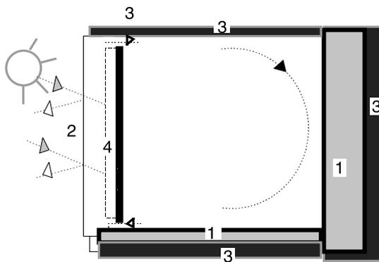
Fig. 16. Indirect – gain system. Standard solar collector wall.
