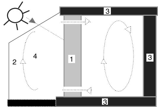
Fig. 17. Sun space coupled with a storage wall.
