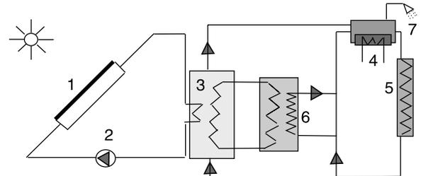
Fig. 10. Series solar-heat pump DHW & space heating.
