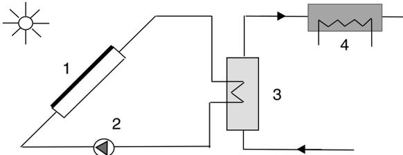
Fig. 4. DHW system with an auxiliary heater.
