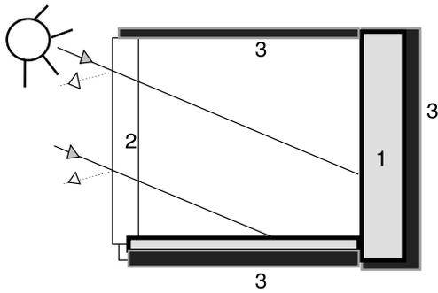
Fig. 13. Direct – gain passive system.
