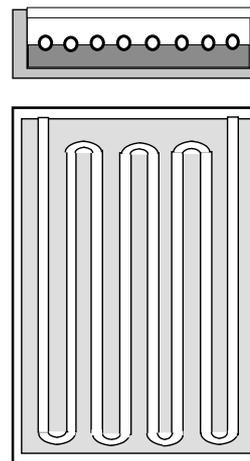
Fig. 1. The cross section and view through the simplified model of a flat plate solar collector.
