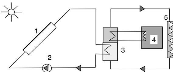
Fig. 7. Space heating with storage coupled with a heater.
