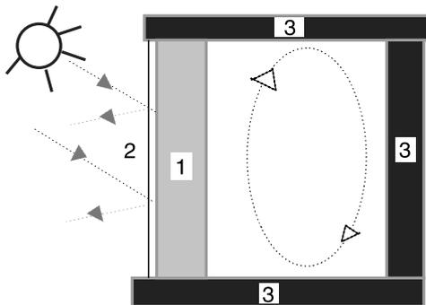
Fig. 14. Indirect – gain system. Solar collector – storage full wall.
