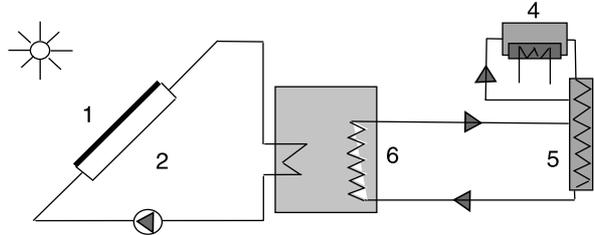
Fig. 11. Parallel solar heat pump space heating system.
