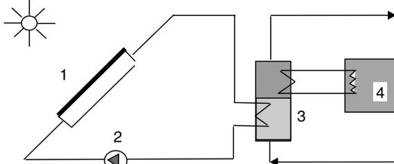
Fig. 5. DHW system with storage coupled with a heater.
