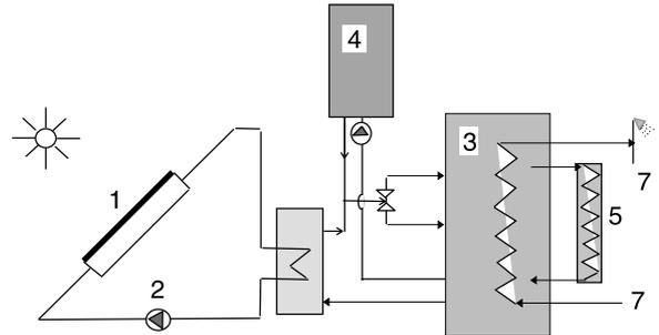
Fig. 8. DHW & space heating with an extra boiler and auxiliary heater.
