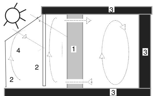
Fig. 19. Double sun space coupled with a storage wall.
