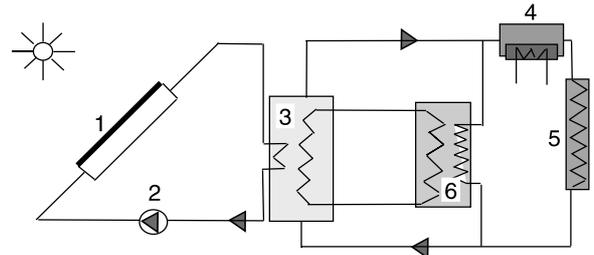
Fig. 9. Series solar-heat pump space heating system.
