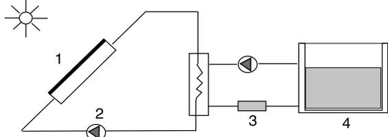
Fig. 3. Close indirect swimming pool system.
