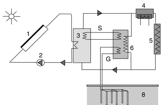
Fig. 12. Double source solar-ground heat pump space heating system.
