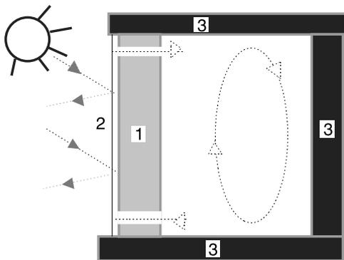
Fig. 15. Indirect – gain system. Ventilated solar collector – storage wall.
