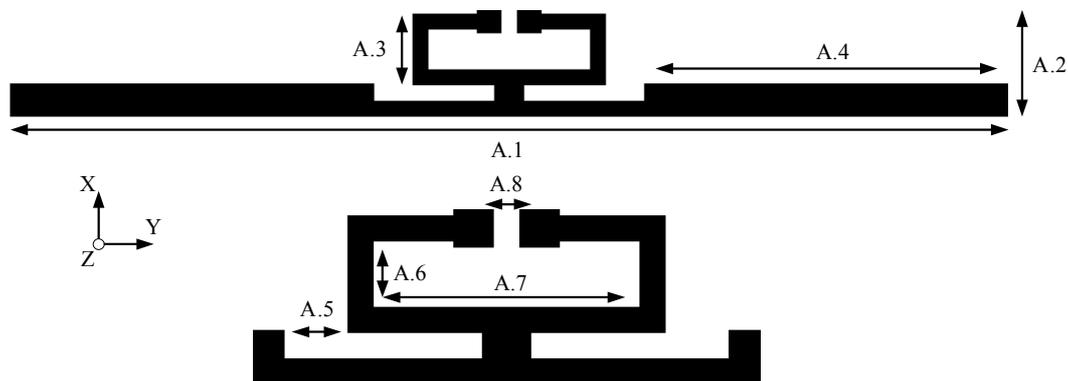
Figure 3. The wide band tag antenna design.
