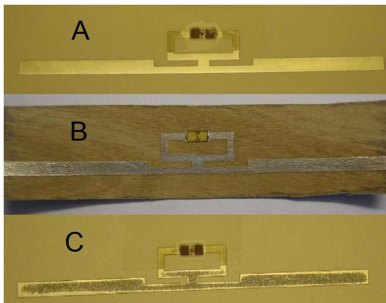
Figure 4. Inkjet-printed tags with ICs on (A) paper; (B) wood; and (C) cardboard.
