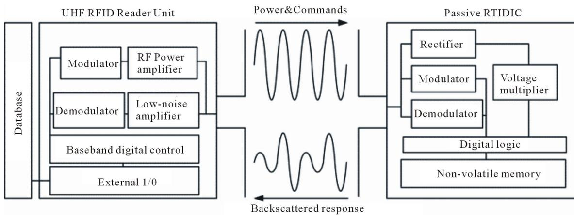
Figure 1. Passive UHF RFID system.
