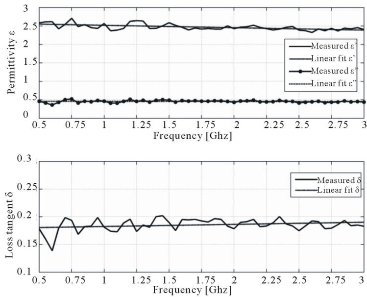
Figure 2. Dielectric properties of the birch based plywood, 23°C and 12% wt.
