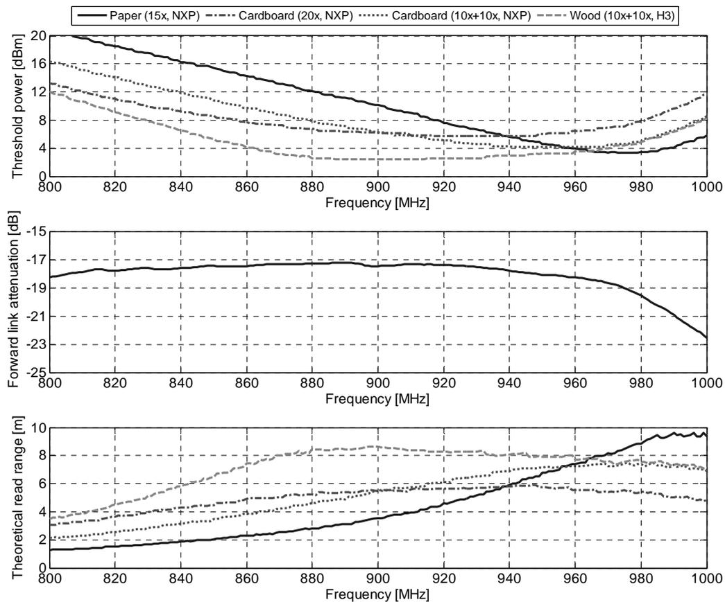
Figure 5. Performance of tags printed on paper, cardboard, and wood.
