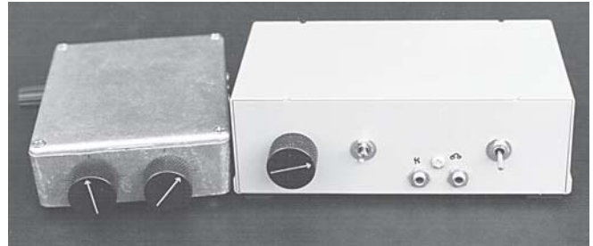
Fig 1.42—Outside view of the Beginner Station. At left is the beginner's direct conversion receiver with the transmitter at the right.
