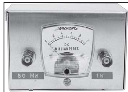
Fig 1.28 —The front panel of the dual-range QRP power meter.
