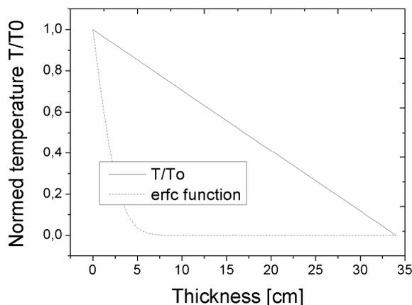
**Figure 2:** The complementary error function of random numbers (1 to 34) and the temperature profile of a given wall
